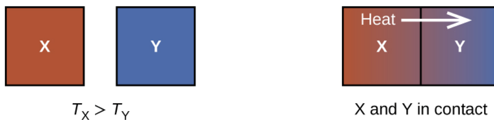
Figure 17.5 When two objects at different temperatures come in contact, heat spontaneously flows from the hotter to the colder object.
