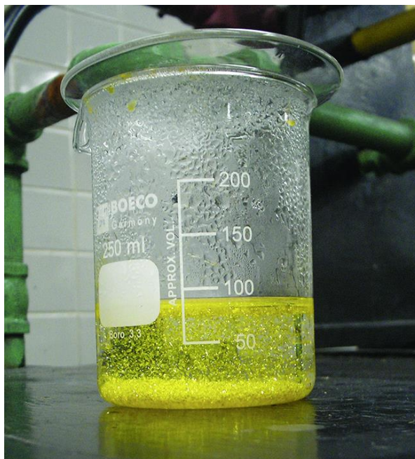
Figure 16.2 A precipitate of \text{PbI}_2 forms when solutions containing \text{Pb}^{2+} and \text{I}^- are mixed. (credit: Der Kreole/Wikimedia Commons)
