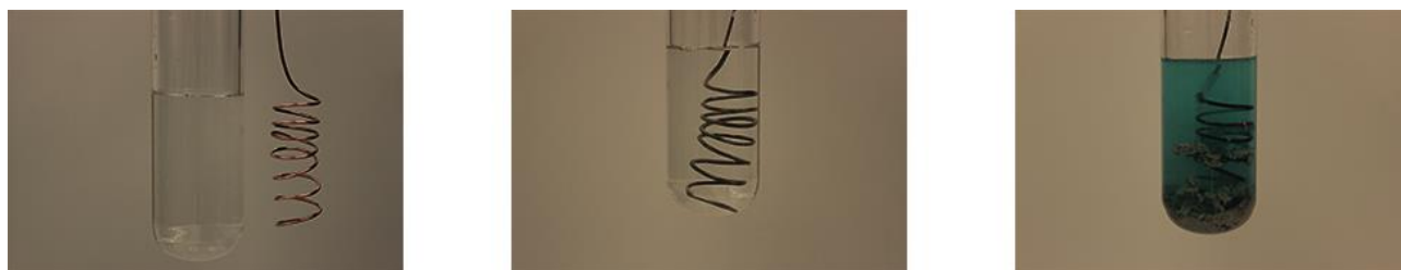
Figure 18.2 A copper wire and an aqueous solution of silver nitrate (left) are brought into contact (center) and a spontaneous transfer of electrons occurs, creating blue \text{Cu}^{2+}(\text{aq}) and gray \text{Ag}(\text{s}) (right).
