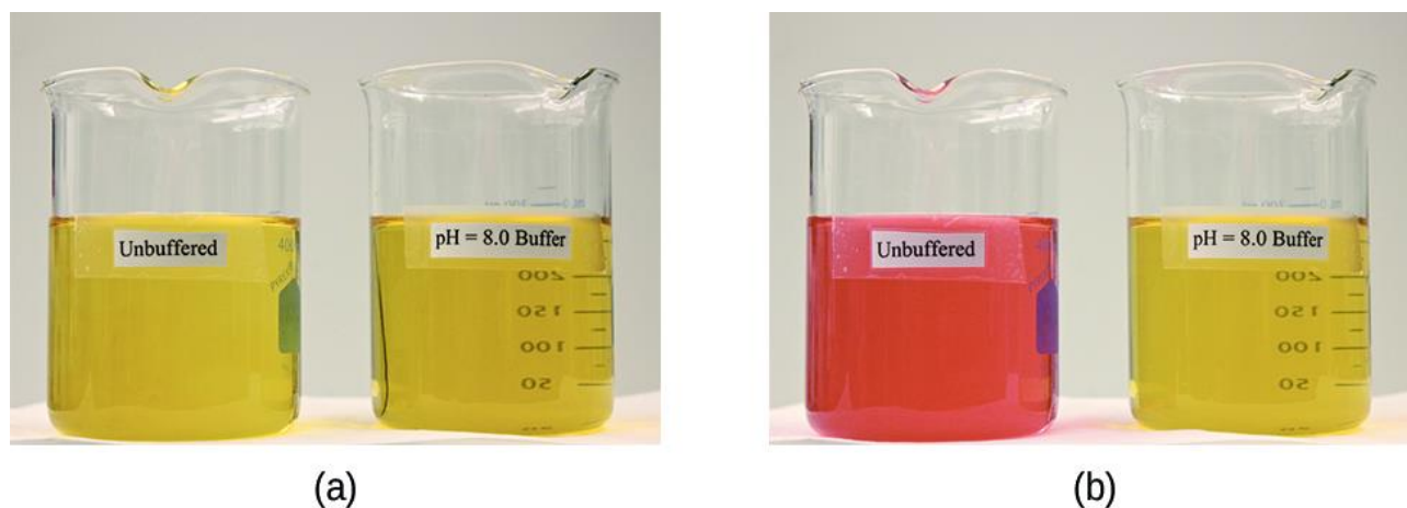
Figure 15.3 (a) The buffered solution on the left and the unbuffered solution on the right have the same pH (pH 8); they are basic, showing the yellow color of the indicator methyl orange at this pH. (b) After the addition of 1 mL of a 0.01- M HCl solution, the buffered solution has not detectably changed its pH but the unbuffered solution has become acidic, as indicated by the change in color of the methyl orange, which turns red at a pH of about 4. (credit: modification of work by Mark Ott)
