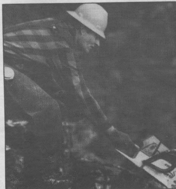
Gary Strom takes one last look to reassure his safety before finishing bucking this tree into log lengths. At the same time he is making sure the log won't slab or tear as the cut is completed.
